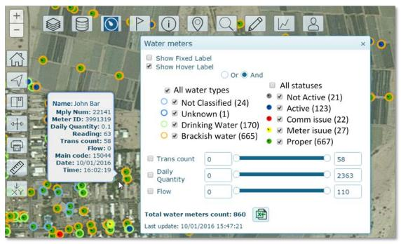
Figure 10: Spatial visualization of water meters- water types and real time consumption and status.
