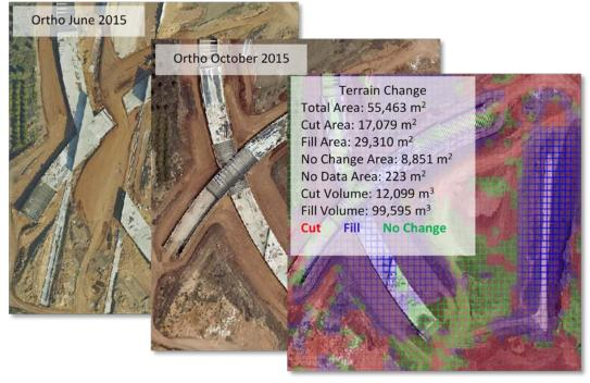
Figure 9: Terrain change monitoring and stock calculation through high resolution orthophoto and detailed DTM.
